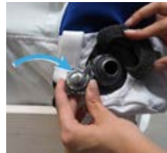
Photo 15: Open front cap of valve.
